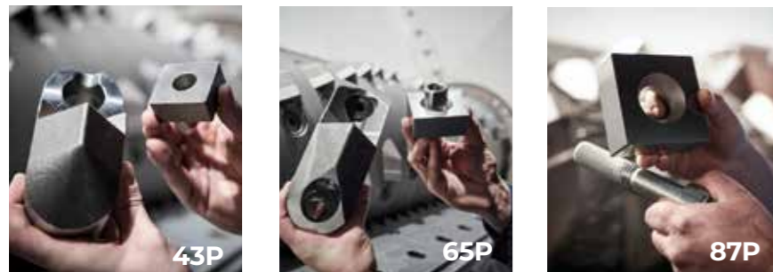
Rotor with pointed knives in 3 knife sizes, four-fold usable
